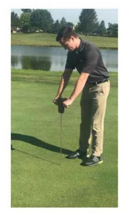
6110FS FieldScout® SC 900 Soil Compaction Meter
